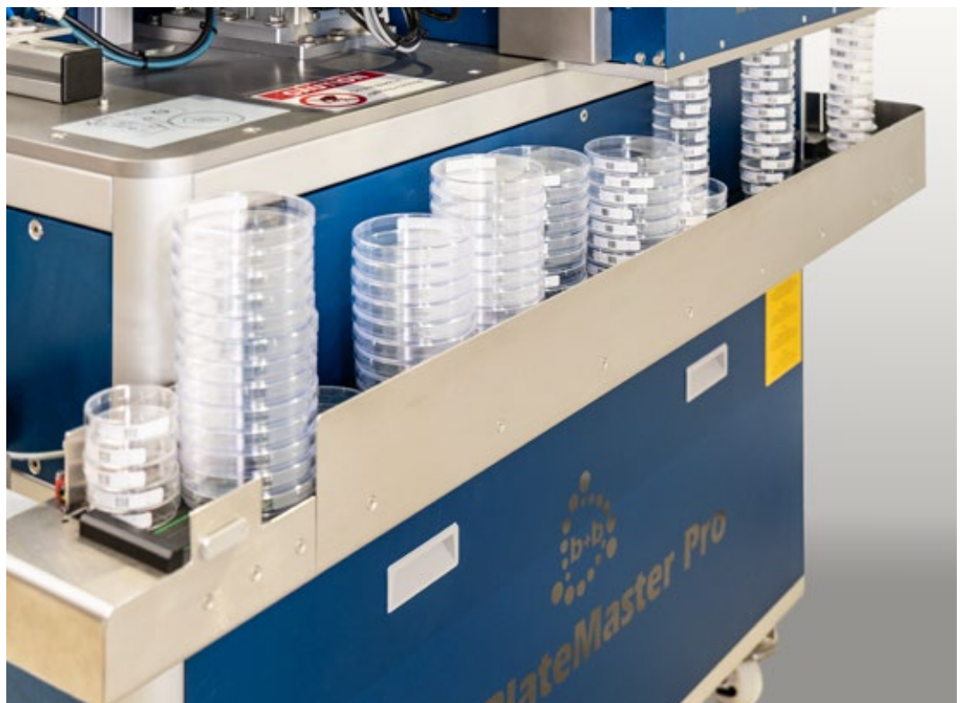
Figure 3: The circulating discharge conveyor transports the stacked Petri dishes to the front of the system
