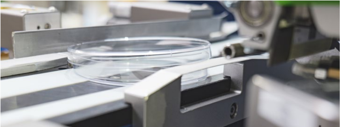
Figure 2: The mechanical lid lifting system for placing the label under (behind) the edge of the lid.
